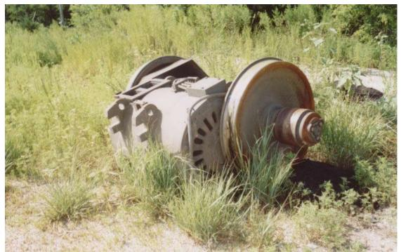
**RAILSCENE:** Power to the rails! Traction motor with gear box and rail wheels typical of the 4 or 6 under modern locomotives all together applying up to 6000 horsepower to the rails. This unit had an enroute malfunction and was replaced.
