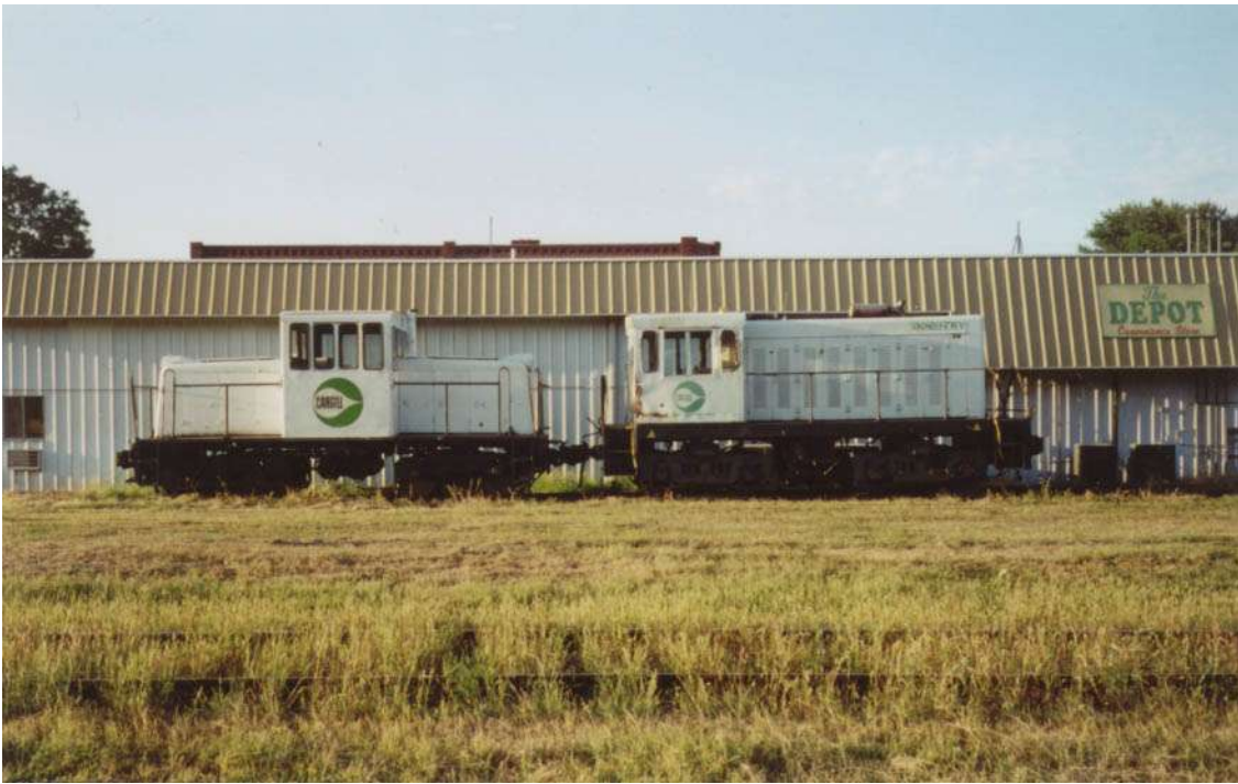
RAILSCENE: Mini-motive power: Two of FEVR's small locomotives in the Hooper yard. 1942 General Electric 45 ton (left) and circa 1955 Baldwin 50 ton (right). These were retired by regional grain elevators and are in good condition.
