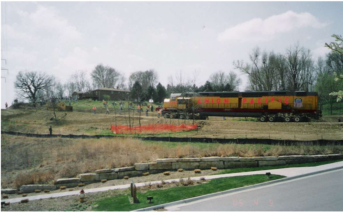
RAILSCENE: Ruling grade: Centennial 6900 ascending the steepest grade of its life, assisted by hydraulically powered rubber tired dollies and a bulldozer , on its way to the new hill-top Kenefick Park. Rail wheels were moved separately.
