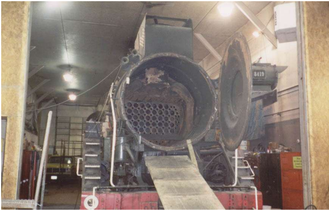
RAILSCENE: Flue Shot! ("shot" as in photo): Open smoke box door on the front of Boone and Scenic Valley JS8419 shows the flues (tubes) which pass hot combustion gases through the boiler from the firebox. (photo with permission)
