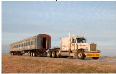
The completed assembly moves on the highway using an approved route assuring that needed clearances and weight capabilities exist. The hours and days of the week that the move is allowed are also specified.
