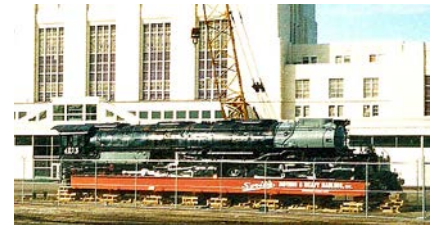
4023 on cribbing before powered road rubber tire wheels are in place. SCRIBBS of David City, NE was the contractor. Durham Museum in the background.
